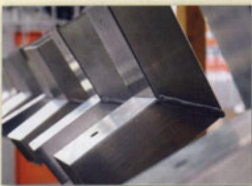
After all treatments, the support is ready to enter the painting cabin, be painted and be taken to the curing oven for the powder to be polymerized.
