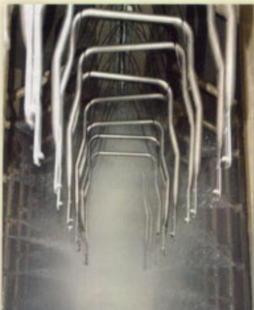
The painting units can process bars up to 3,300 mm in length. The overall dimensions for manufactured goods are 3,000 mm in length, 1,400 mm in height, 800 mm in width.
